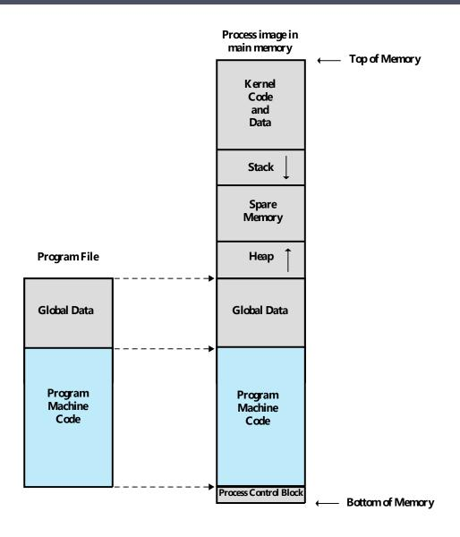
Figure 10.4 Program Loading into Process Memory
